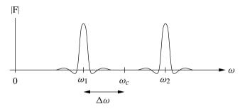
The bandwidth of the periodic FSK signal is then  $2\Delta f + 2B$ , with B the bandwidth of the baseband signal.
