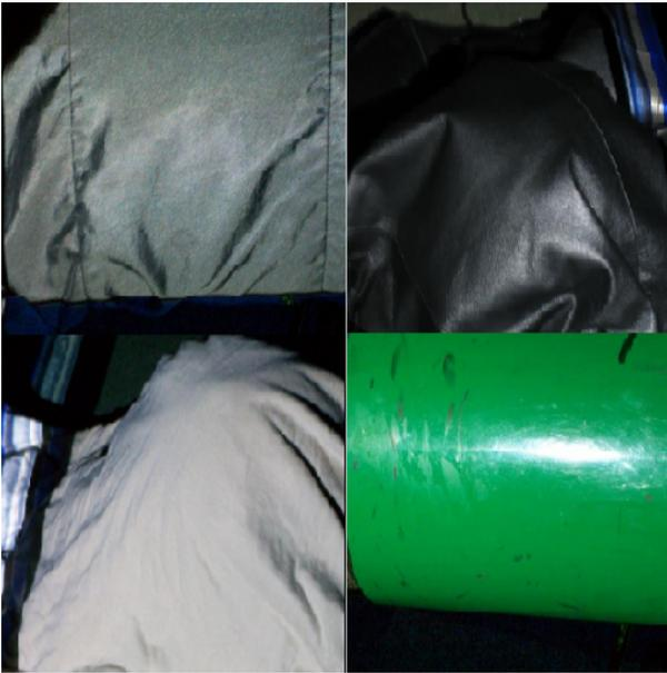
Figure 4. Surfaces 1 to 4 of twelve used to test the BRDF based classification power of the PMC developed sample sets. Each material was reconstructed and its BRDF calculated four times using our PMC based parameter estimation method.
