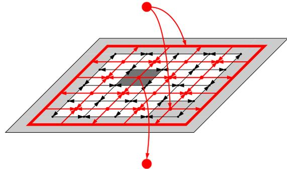
Figure 3. Graph construction for 2D segmentation. Dual arcs linking to displayed (dual) nodes all have infinite weight. The dark region is constrained to the interior via an infinite arc to the sink. Light regions (including the exterior face region) are constrained to the exterior via an infinite arc from the source. Other arcs between dual nodes (red) and terminal nodes are not shown.
