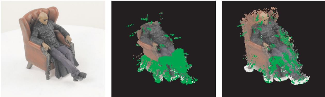
(a) One of 8 images used in reconstruction. (b) Minimum surface (no ballooning): ratio=647.4. (c) Ratio surface: ratio=258.6.
