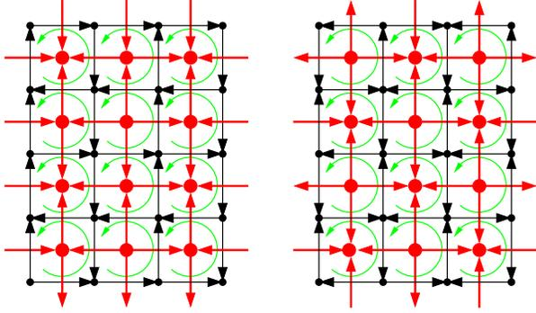
Figure 2. Possible oriented 2D meshes for use in minimum ratio cut. Oriented boundaries are composed of directed edge elements (black arrows), which are in one-to-one correspondence with dual edges (red arrows).
