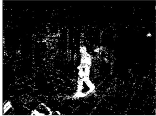
FIGURE 1: Thresholded background subtraction. The foreground pixels are highlighted.
