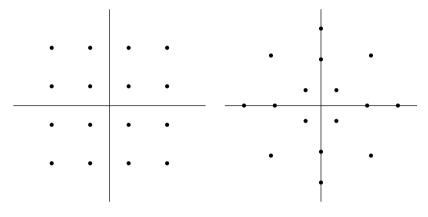
The first uses three different amplitudes, two with four phases and one with eight. The second uses four amplitudes and four phases.
