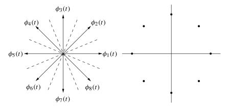
All signals have the same energy  $E_s$  over the interval  $(0, T_s)$ , and each signal is correctly demodulated at the receiver if the phase is within  $\pm \pi/M$  of the correct phase  $\theta_i$ . No information is contained in the energy of the signal.
