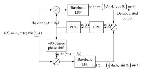
This can be analysed by assuming that the VCO is locked to the input suppressed carrier frequency  $f_c$ , with a constant phase error of  $\theta_e$ . Then the voltages  $v_1(t)$  and  $v_2(t)$  are obtained at the output of the baseband lowpass filters as shown. Since  $\theta_e$  is small, the amplitude of  $v_1(t)$  is relatively large compared to that of  $v_2(t)$ . Furthermore,  $v_1(t)$  is proportional to m(t), so it is the demodulated output. The product voltage  $v_3(t)$  is
