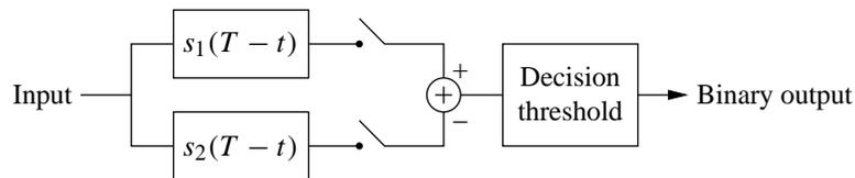
The first filter is matched to the signal  $s_1(t)$ , and the second to  $s_2(t)$ . Under the assumption that the signals are mutually orthogonal, the output of one of the matched filters will be  $E$  and the other zero (where  $E$  is the energy of the
