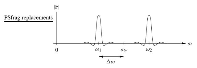
The bandwidth of the periodic FSK signal is then  $2\Delta f + 2B$ , with B the bandwidth of the baseband signal.
