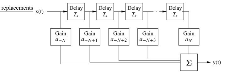
As shown, the transversal filter consists of a tapped delay line where the tap outputs are multiplied by gain factors. The resulting products are summed to produce the filter output. The transversal structure is popular for this application because it is easy to analyse and design, and has efficient means of implementation. The input x(t) is from the channel, and the equaliser is designed to provide an output waveform y(t) that has zero ISI.
