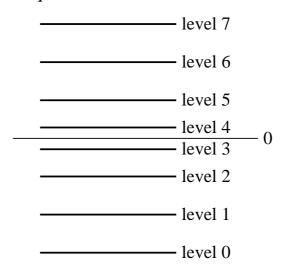
More often, nonuniform quantisation is achieved by first distorting the original signal with a nonlinear **compressor** characteristic, and then using a uniform quantiser on the result:
