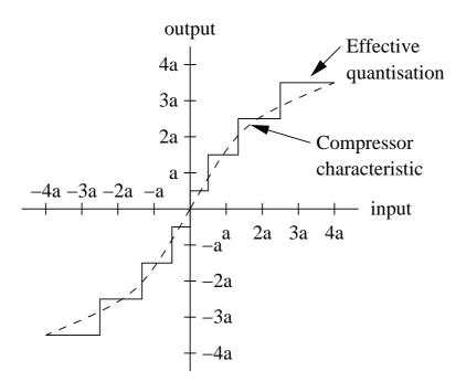
A given signal change at small magnitudes will then carry the uniform quantiser through more steps than the same change at large magnitudes. At the receiver, an inverse compression characteristic (or **expansion**) is applied, so that the overall transmission is not distorted. The processing pair (compression and expansion) is usually referred to as **companding**.
