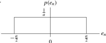
The average value of this error is zero, owing to the symmetry of the probability density. The mean square error (MSE) is
