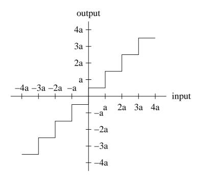
The signal is mapped through this function prior to being sampled.
