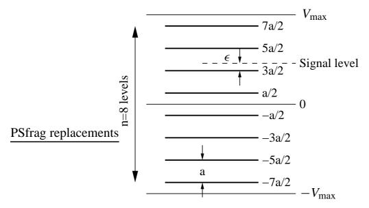
Equivalently, the quantisation operation can be considered in terms of an input-output relation of the form:
