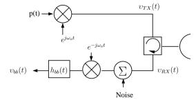
(a) Draw a block diagram of a physical implementation of this radar showing an I/Q up-converter, an I-Q down-converter, and appropriate sampling into a digital signal processing computer.
