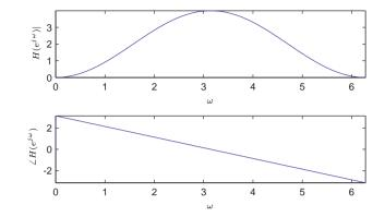
DC is the only frequency that is completely blocked.
