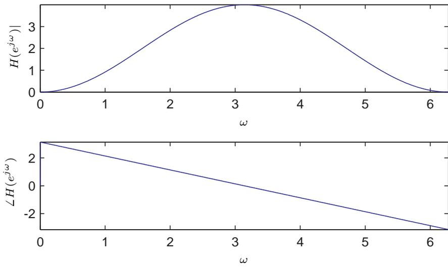
DC is the only frequency that is completely blocked.
