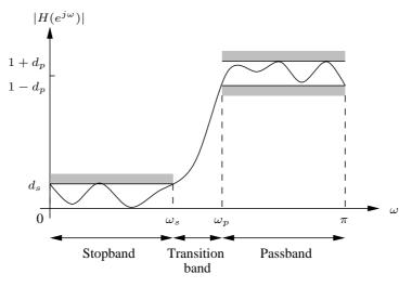
For a sampling rate of 48kHz the highest frequency that can be represented is 24kHz, and this corresponds to  $\omega = \pi$  rad/sample.
