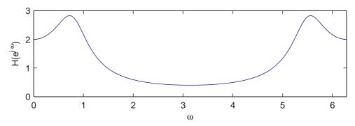
(c) For a 12kHz sampling rate the Nyquist frequency is 6kHz and corresponds to  $\omega = \pi$ . The discrete frequency  $\omega = \pi/4$  therefore relates to 6/4 = 1.5kHz, and this is the center frequency of the analog system.
