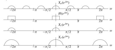
The lowpass filter  $H(e^{j\omega})$  as drawn has a cutoff frequency of  $\pi/6$ , but any cutoff in the range  $\pi/6$  to  $\pi/2$  will meet the filtering requirements.
