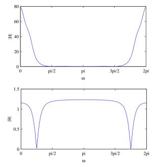
The numbers in these plots are for poles at  $0.8e^{\pm j\pi/6}$  and 0.8 in the first case, and  $0.8e^{\pm j\pi/4}$  in the second. However, Since no numbers were given I cannot expect numerical correctness — all that is required is the basic characteristics.
