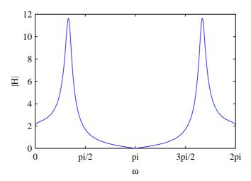
The filter has a bandpass characteristic, with the response peaking at around  $\omega = \pi/3$  (passes low frequencies, amplifies frequencies around  $\pm \pi/3$ , and attenuates high frequencies).
