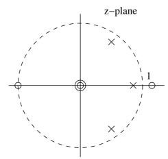
What type of filter does this system represent? What is the approximate phase response of the system at  $\omega = 0$ ?
