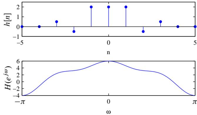
Recall from the properties of the Fourier transform this filter has a real-valued frequency response  $A(e^{j\omega})$ . Delaying this impulse response by  $(N - 1)/2$  results in a causal filter with frequency response
