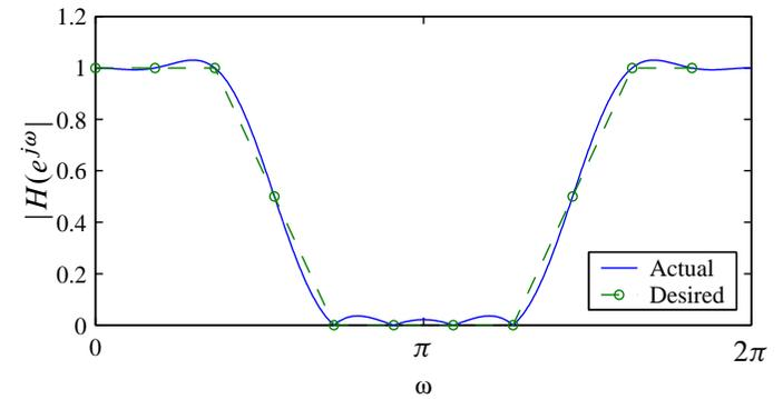
By leaving the value of the transition sample unconstrained, one can to some extent optimise the filter to minimise the ripple. Empirically, with three transition samples a stopband attenuation of 100dB is achievable. Recall however that for  $h[n]$  real we require even or odd symmetry in the impulse response, so the values are not entirely unconstrained.
