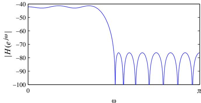
The maxima and minima are known as extrema. For linear phase lowpass filters, for example, there are either  $r + 1$  or  $r + 2$  extrema, where  $r = (N + 1)/2$  (for type 1 filters) or  $r = N/2$  (for type 2 filters).
