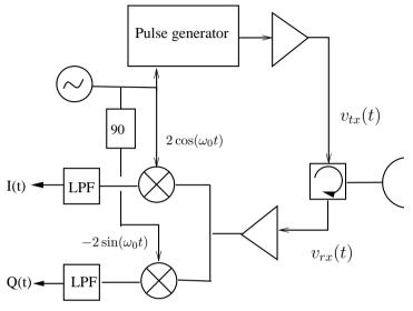
(a) Draw a neatly labelled block diagram of an equivalent analytic signal model of the radar.
