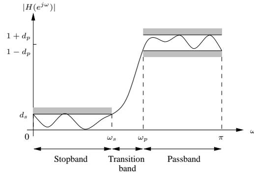
For a sampling rate of 48kHz the highest frequency that can be represented is 24kHz, and this corresponds to  $\omega = \pi$  rad/sample.
