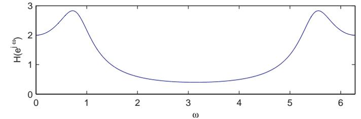
(c) For a 12kHz sampling rate the Nyquist frequency is 6kHz and corresponds to  $\omega = \pi$ . The discrete frequency  $\omega = \pi/4$  therefore relates to  $6/4 = 1.5$ kHz, and this is the center frequency of the analog system.
