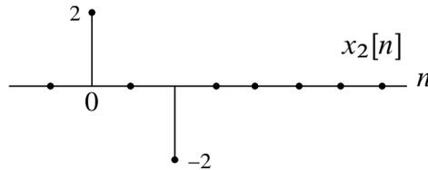
The response to  $x[n]$  is  $y[n]$ . Since the system is LTI, the response to  $2x[n]$  is  $2y[n]$  and the response to  $-2x[n-1]$  is  $-2y[n-1]$ . But observe that the signal  $x_2[n]$  is just  $2x[n] - 2x[n-1]$ , so the output must be the sum  $2y[n] - 2y[n-1]$ .
