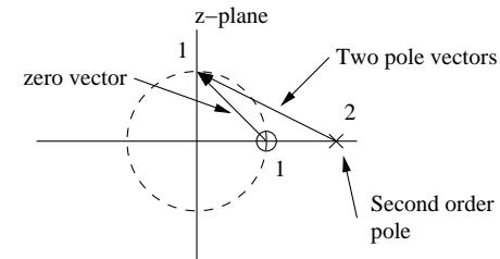
$$\text{Gain} = \frac{\prod \text{length of zero vectors}}{\prod \text{length of pole vectors}} = \frac{\sqrt{1^2 + 1^2}}{\sqrt{1^2 + 2^2}\sqrt{1^2 + 2^2}} = \frac{\sqrt{2}}{5}.$$
