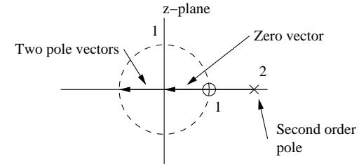
$$\text{Gain} = \frac{\prod \text{length of zero vectors}}{\prod \text{length of pole vectors}} = \frac{2}{(3)(3)} = \frac{2}{9}.$$
