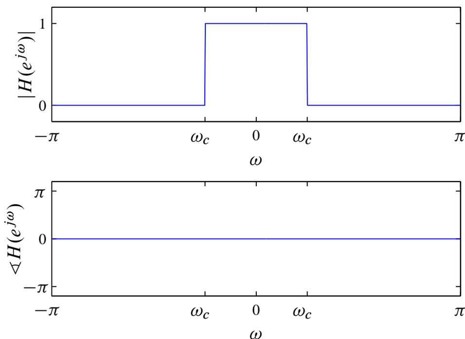
This response, as for all discrete-time signals, is periodic with period  $2\pi$ . Its impulse response (for  $-\infty < n < \infty$ ) is
