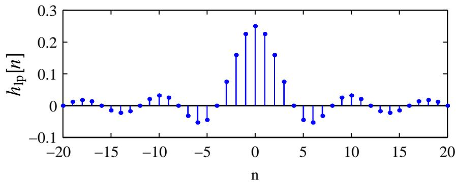
The ideal lowpass filter is noncausal, and its impulse response extends from  $-\infty < n < \infty$ . The system is therefore not computationally realisable. Also, the phase response of the ideal lowpass filter is specified to be zero — this is a problem in that causal ideal filters have nonzero phase responses.
