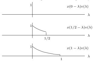
(b) The convolution output for the three points specified is the area under the three curves given above. Thus w(0) = 0, and
