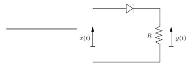
Assume an ideal diode with zero forward voltage drop.
