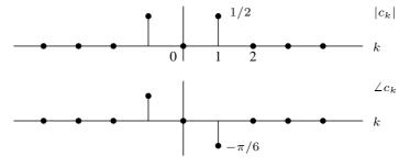
(b) The trigonometric Fourier series requires  $\omega_0 = 3\pi$  and the coefficients satisfy  $a_0 = c_0 = 0$ ,  $a_1 = 2|c_1| = 1$  and  $b_1 = \angle c_1 = -\pi/6$ , with all other coefficients  $a_k$  and  $b_k$  zero.
