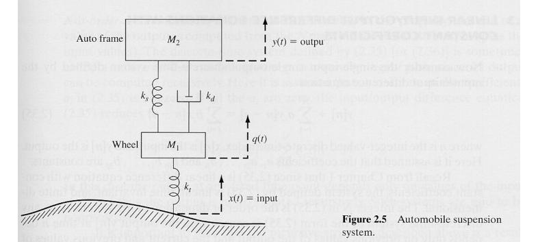
$$\begin{cases} M_1 \frac{d^2 q(t)}{dt^2} + k_t [q(t) - x(t)] = k_s [y(t) - q(t)] + k_d \left[ \frac{dy(t)}{dt} - \frac{dq(t)}{dt} \right] \\ M_2 \frac{d^2 y(t)}{dt^2} + k_s [y(t) - q(t)] + k_d \left[ \frac{dy(t)}{dt} - \frac{dq(t)}{dt} \right] = 0 \end{cases}$$
