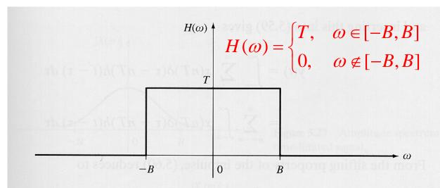
Figure 5.25 Frequency response function of ideal lowpass filter with bandwidth B.
