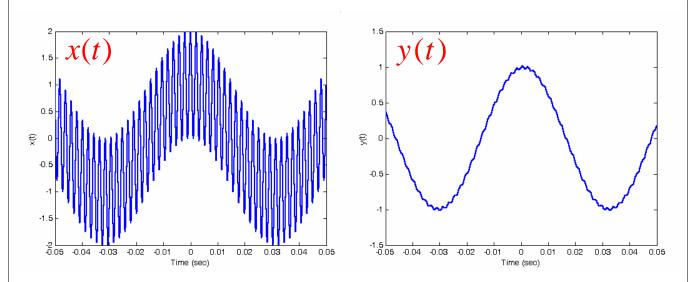
The RC circuit behaves as a lowpass filter, by letting low-frequency sinusoidal signals pass with little attenuation and by significantly attenuating high-frequency sinusoidal signals
