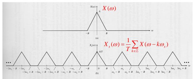
Figure 5.24 Fourier transform of (a) x(t) and (b)  $x_s(t) = x(t)p(t)$ .
