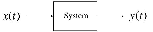
If the input signal is x(t) = δ(t) and the system has no energy at t = 0<sup>-</sup>, the output y(t) = h(t) is called the impulse response of the system
