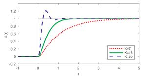
We see that the response for K = 7 is quite slow, and the system takes a long time to reach the setpoint. The response for K = 80 is much faster, but this comes at the cost of overshoot and ringing. The case of K = 16 yields the fastest response without oscillations.
