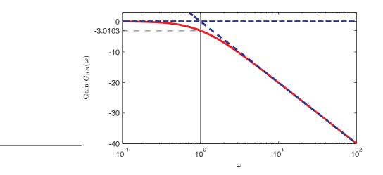
Also shown are dotted (blue) asymptotes to the curve. Firstly, for  $\omega \ll \omega_c$  the gain is approximately  $G_{\rm dB}(\omega) \approx -20 \log_{10}(\sqrt{1}) = 0$ . This is the horizontal asymptote in the plot. Secondly, for  $\omega \gg \omega_c$  the ratio  $\omega/\omega_c \gg 1$  and  $\sqrt{1 + (\omega/\omega_c)^2} \approx \sqrt{(\omega/\omega_c)^2} = \omega/\omega_c$ , so the gain is approximately
