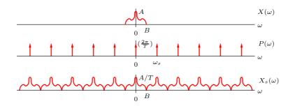
The signal x(t) can just be reconstructed from the samples x[n], although to do this we do need a perfect reconstruction filter.
