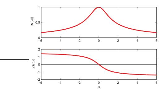
This is called the *Bode plot* of the system (although typically Bode plots are displayed on logarithmic axes, as will be shown shortly).
