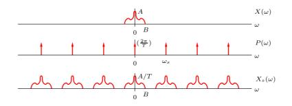
The signal  $X_s(\omega)$  can be seen to contain *replicas* of the signal  $X(\omega)$  at integer multiples of the sampling frequency  $\omega_s = \frac{2\pi}{T}$ . In the case drawn above we have  $\omega_s > 2B$ , and the replicas are not overlapping. Evidently we can then recover  $X(\omega)$  from  $X_s(\omega)$  by passing it through a filter with the following frequency response:
