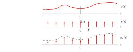
The interesting fact is that x(t) can be recovered from  $x_s(t)$  as long as x(t) is appropriately bandlimited. Suppose B is the highest frequency present in x(t), so  $X(\omega) = 0$  for  $|\omega| > B$ . An impulse train in time corresponds to an impulse train in frequency, so
