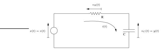
The input is the voltage generated by the voltage source on the left, and the output is the voltage across the capacitor on the right.
