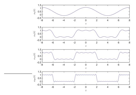
Small values of N yield a poor reconstruction, but as N increases the reconstructed signal tends towards the original signal x(t).
