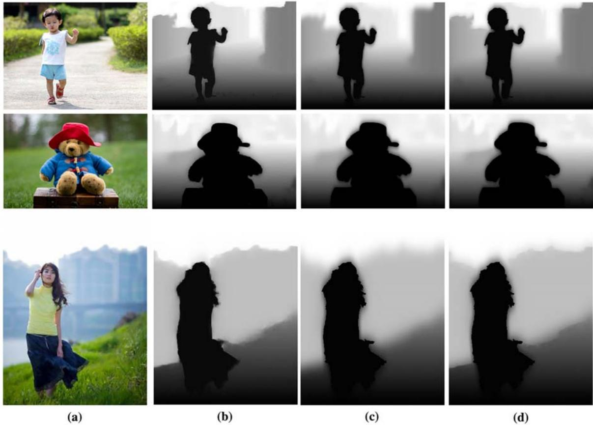
**Fig. 86 Gradient-based depth maps. (a) Original images; (b) Depth maps; (c) Asymmetrically smoothed depth maps; (d) Final merged asymmetrically smoothed depth maps.**
