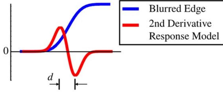
Fig. 46 Model for distance between second-derivative extrema [60]
