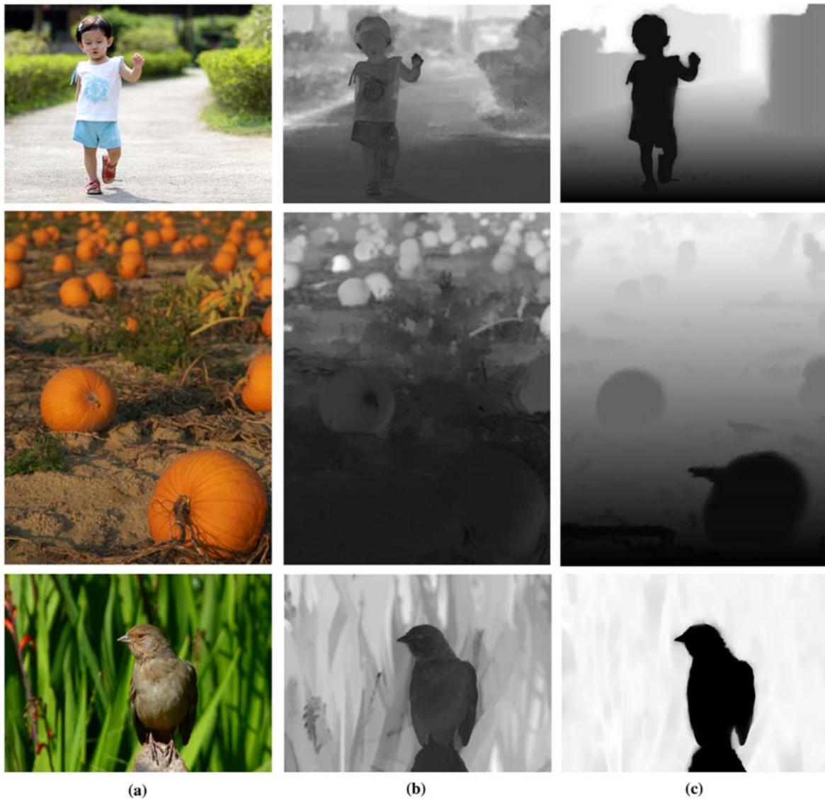
**Fig. 56 Benchmarking: *Kid*, *Pumpkin* and *Bird-Reed* (from top to bottom). (a) Original image; (b) Defocus map generated by Zhou and Sim [63]; (c) Depth map generated using proposed method.**
