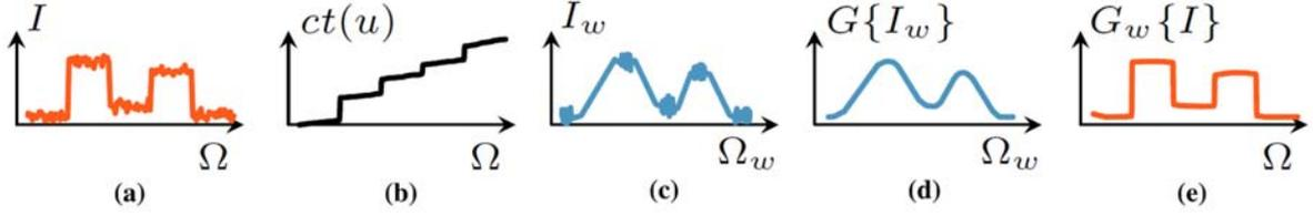
**Fig. 51 Domain transform edge-aware filtering [133]. (a) Input signal  $I$  in original domain; (b) Associated domain transform;  $ct(u)$ ; (c)  $I$  in the transformed domain; (d) Filtering using a Gaussian filter in the frequency domain; and (e) Filtered signal obtained through the reversal of  $ct(u)$  for  $G\{I_w\}$ .**
