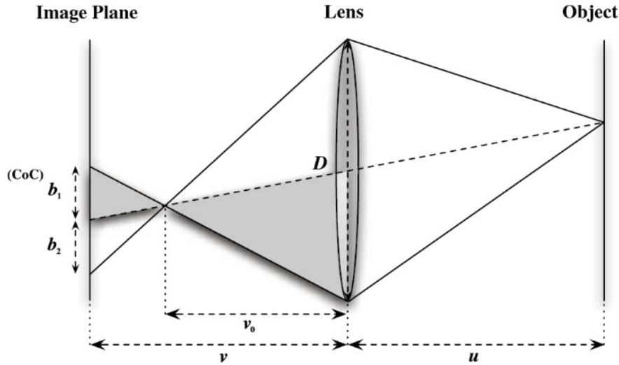
**Fig. 43 Geometry of (real) finite-aperture imaging system [121]**
