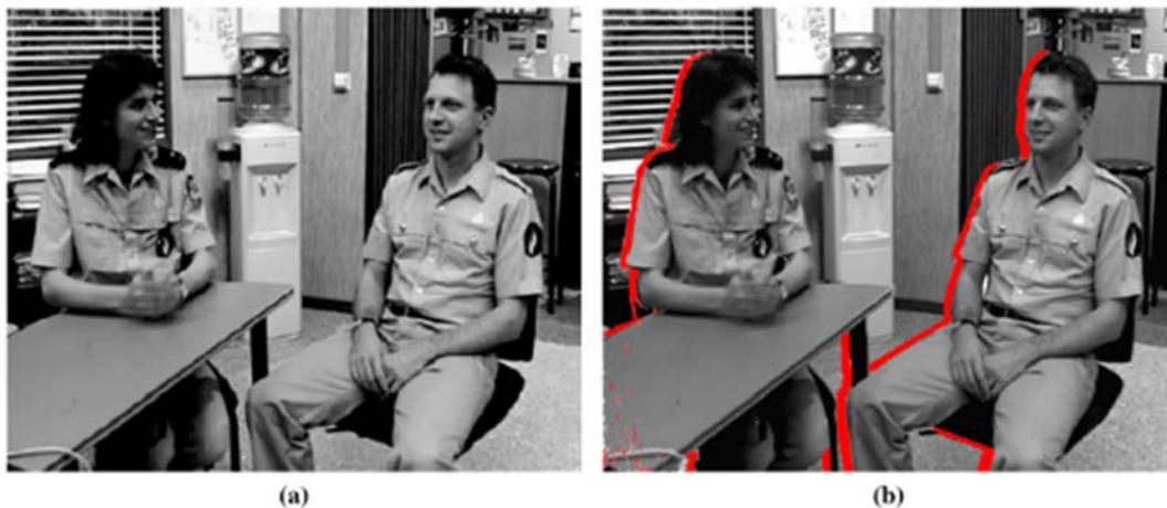
**Fig. 83 DIBR Image Warping [47]. (a) Original image; (b) Warped “Left-view” image (The red indicates the dis-occluded regions).**
