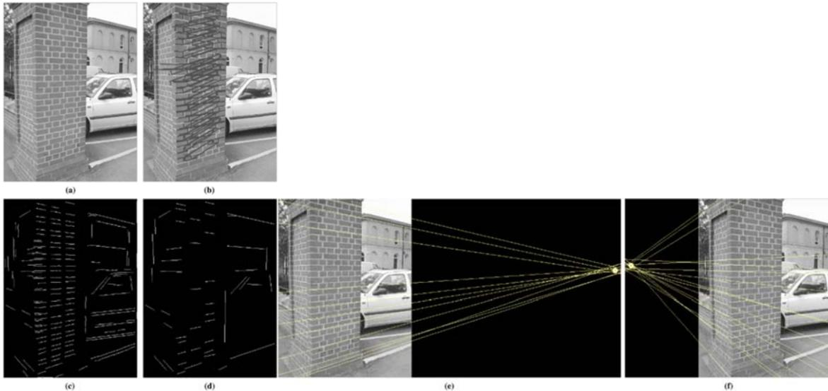
**Fig. 73 Training set 2. (a) Original image; (b) Incorporation of coplanar parallel lines using the feature extraction method proposed by Schaffalitzky and Zisserman [59]; (c) Extracted straight edges using the proposed method; (d) Refined straight edges using the proposed method; (e) Results of the proposed method (Dominant VP); (f) Results of the proposed method (Secondary VP).**
