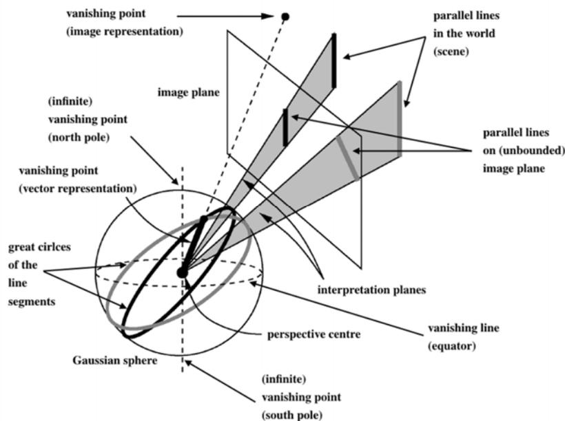
Fig. 64 Gaussian-sphere as an accumulator space [154].
