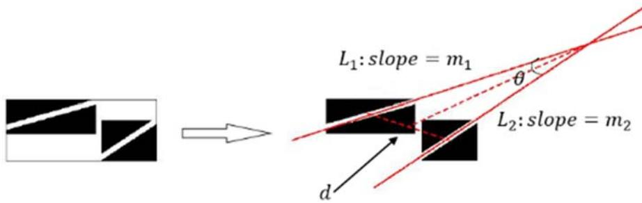
**Fig. 65 Object combination scheme for two regression lines [140]**
