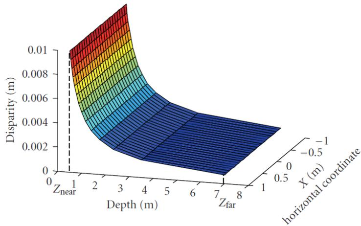
Fig. 81 Relationship between disparity, depth and horizontal position for sample parallel cameras ( $t_c = 0.1$  m and  $f = 0.05$  m) [168].
