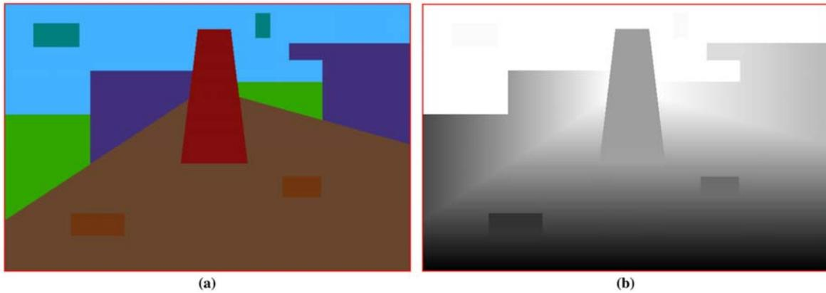
**Fig. 55 Relative depth assignment. (a) Gestalt regions. Brown indicates the ground region, green and purple indicates the peripheral ground objects, the OOI is displayed in maroon and the sky region is indicated in blue; (b) Associated depth map. This shows the depth values of the peripheral ground objects following the contours of the ground. The OOI represents an object on top of the ground; therefore, the entire OOI region is assigned the same relative depth value.**
