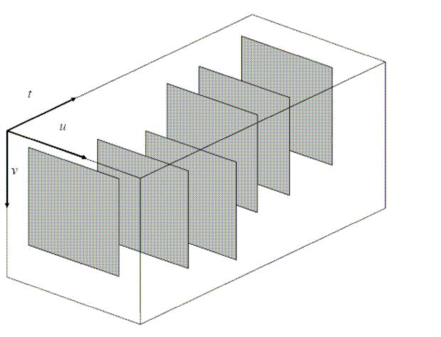
**Figure 5.1: Temporal Alignment:** in the absence of parallax, a temporal line through the image planes corresponds to the same world point.
