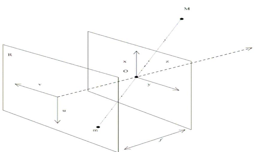
Figure 2.1: The perspective Camera Model
