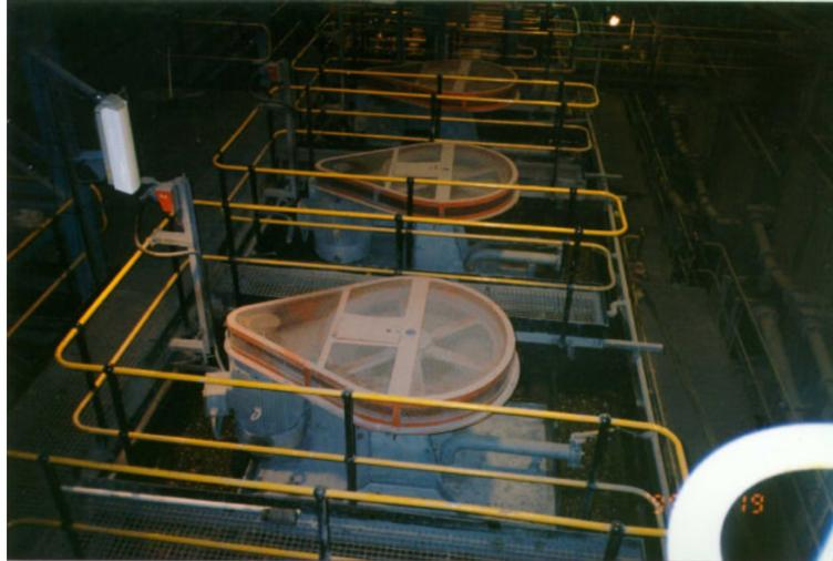
Figure 9.11: A camera installation on a flotation cell
