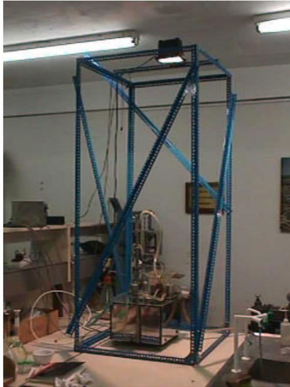
Figure 9.2: Camera support assembly for batch flotation tests
