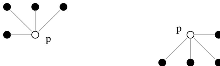
Figure 5.11:  $N_G^+(p)$  and  $N_G^-(p)$  in 8-connectivity
