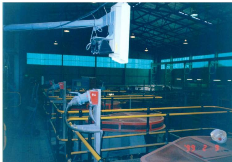
Figure 9.12: A more detailed view of the camera and floodlight assembly
