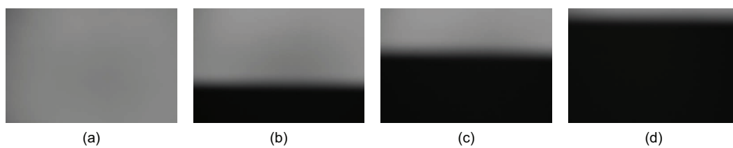
Figure 3.12: Photographs showing the adverse effects encountered when combining time-varying lighting and curtain shutters. In each instance a grey card was illuminated near the end of a 1/60 s exposure time, specifically 4.3ms, 3.0ms, 2.3ms and 1.7ms from the end respectively.
