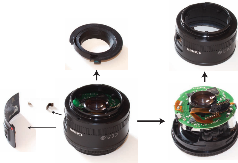
Figure B.2: Photograph showing lens disassembly. Step 2: Removal of mounting bracket and side panel, and separation of inner and outer tubes.
