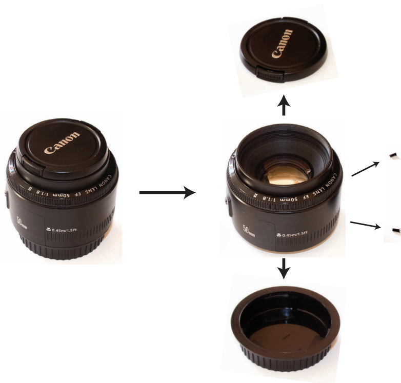
Figure B.1: Photograph showing lens disassembly. Step 1: Removal of front and rear caps, and removal of two micro-screws from mounting bracket.
