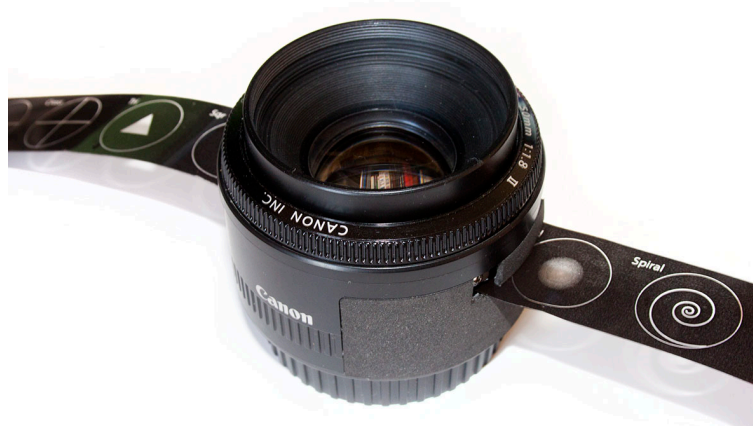
Figure 3.4: A photograph of the modified lens, showing the slots cut into the body to allow the aperture strip to be inserted.
