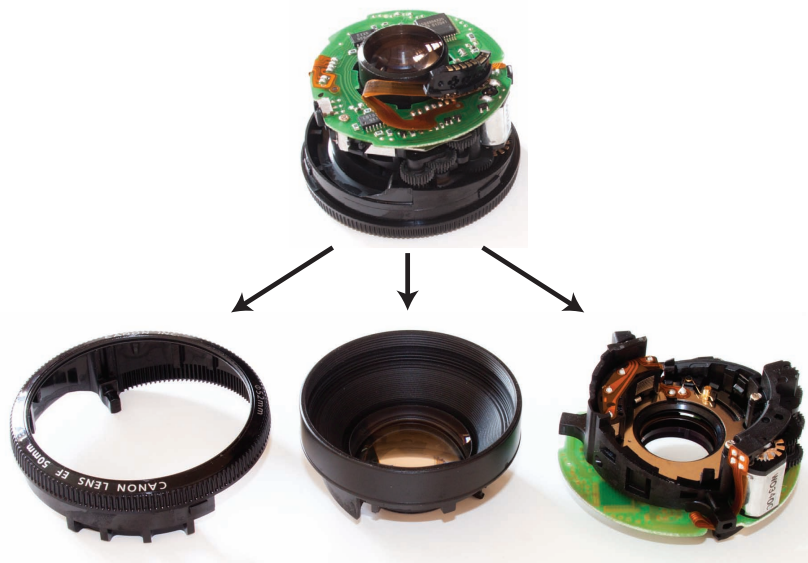
Figure B.3: Photograph showing lens disassembly. Step 3: Separation of inner-tube into focus adjustment ring, front optical element, and aperture plane.
