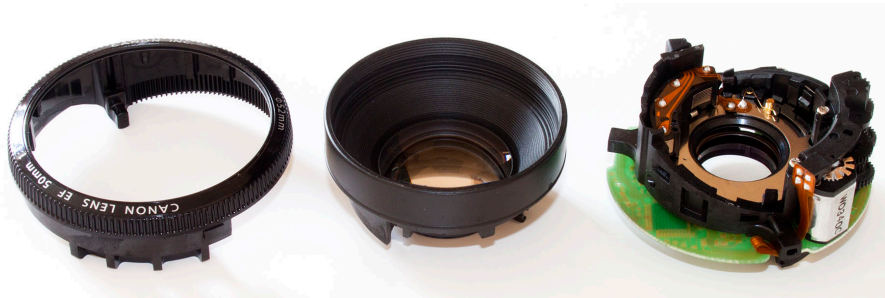
Figure 3.2: A photograph showing the particular stage in the lens disassembly where the front optical element was separated from the aperture module.
