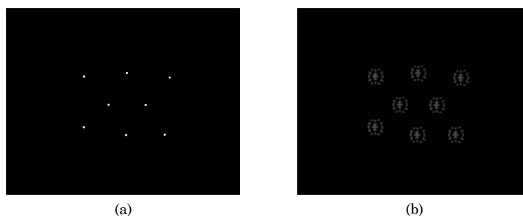
Figure 6.10: An example image pair that was as input to the aperture calibration algorithm. (a) A sharp image of the calibration dots. (b) The observed blurred image.
