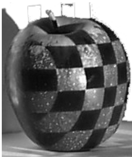
Figure 1.2: Chessboard pattern projected onto an apple to show three-dimensional surface characteristics of the fruit by means of analysing the distortions of the grid pattern on the fruit's surface.
