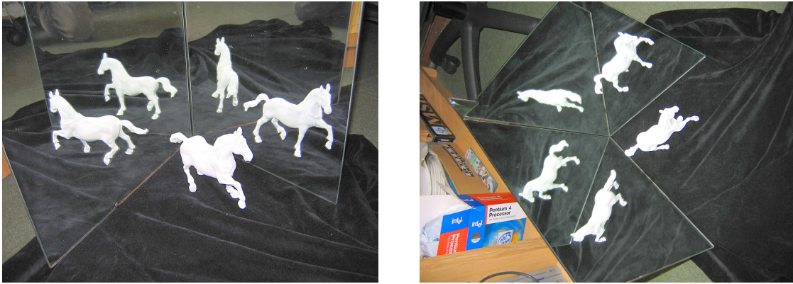
Figure 4.2: Two images of a two-mirror setup positioned so that five views of the object can be seen. Note that the camera has moved between shots, but the mirrors and object have not moved.
