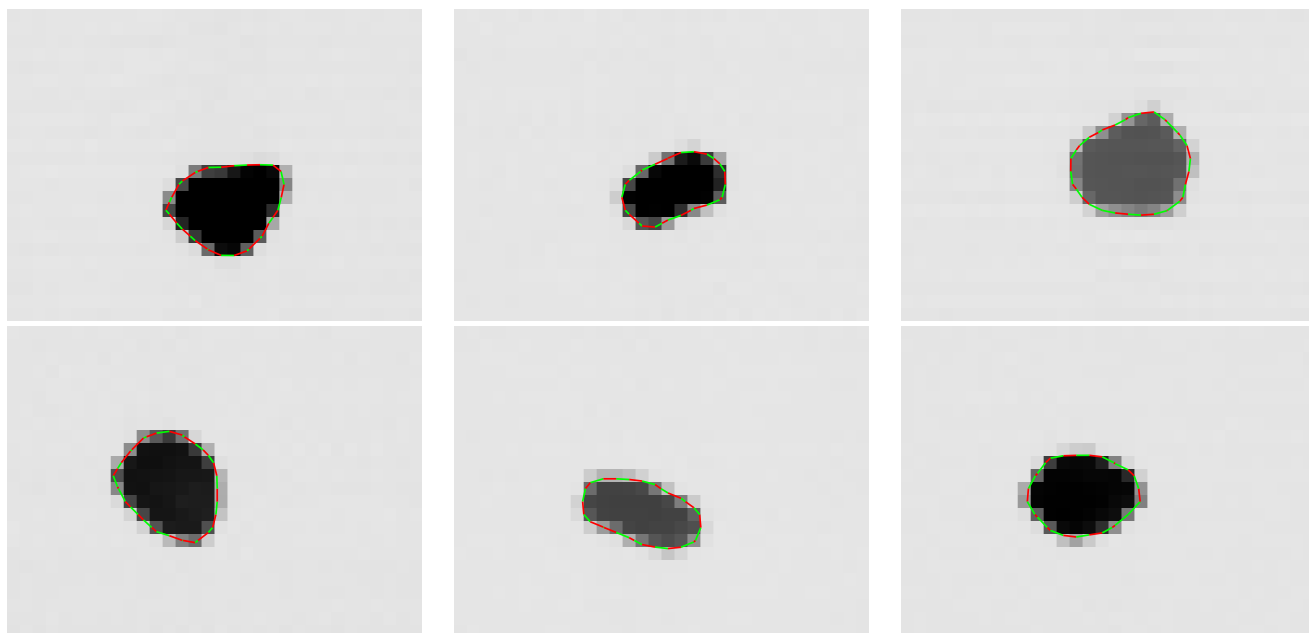
Figure 7.11: An example of a six-view image set of a garnet after 32 \times 32 downsampling. Extracted polygonal boundaries are shown in colour.
