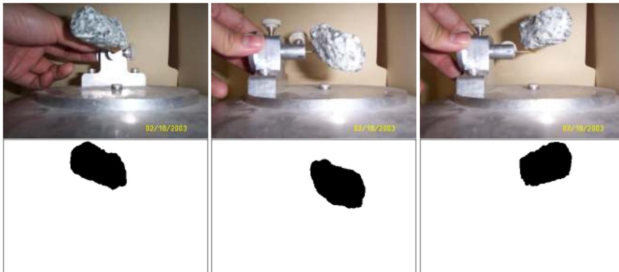
**Figure 2.3:** Three images from a sequence captured using a turntable device for rotating individual rocks about two different axes (*top row*), and the corresponding manually segmented silhouettes (*bottom row*) (pictures from Lau [72]). The images were used to investigate volume prediction from multiple silhouette views.
